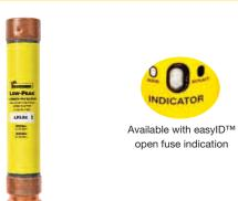
**Description:** Ultimate protection Class RK1 dual element, current-limiting, time-delay fuses available with optional open fuse indication on select ratings. Time-delay – 10 seconds (minimum) at 500% of rated current.
